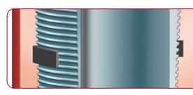
(Option) **SUPERMAX-TSR** Resilient seal for high gas pressure application
